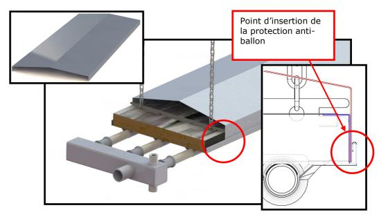
**Figure 3.28**Position des protections anti ballons.
